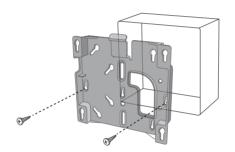
Securing the antenna to the mounting plate
